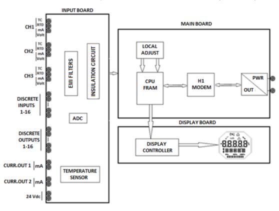
Figure 1.1 – Block diagram for VIO10-P.
