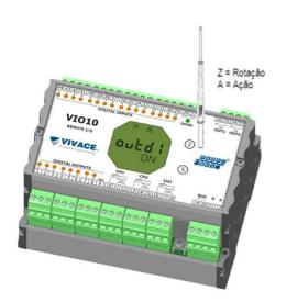
Figure 3.1 shows Z and S markings for local configuration, stamped on device enclosure tag and their functions on magnetic screwdriver actuation.
