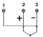
Figure 2.5 - TC or millivoltage connection.
