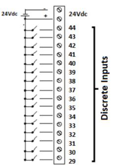
Figure 2.8 – Discrete input connections.
