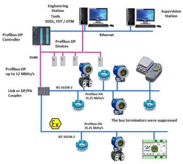
Figure 2.10 - Connection of Profibus-PA devices on the Profibus network.
