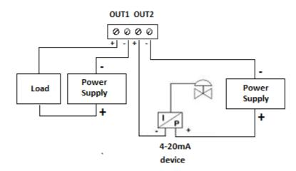
Figure 2.6 – Connection between 4-20 mA output and I/P device or discrete action.
