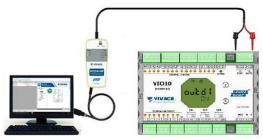
Figure 3.5 – Connection of VCI10-UP to VIO10-P.
