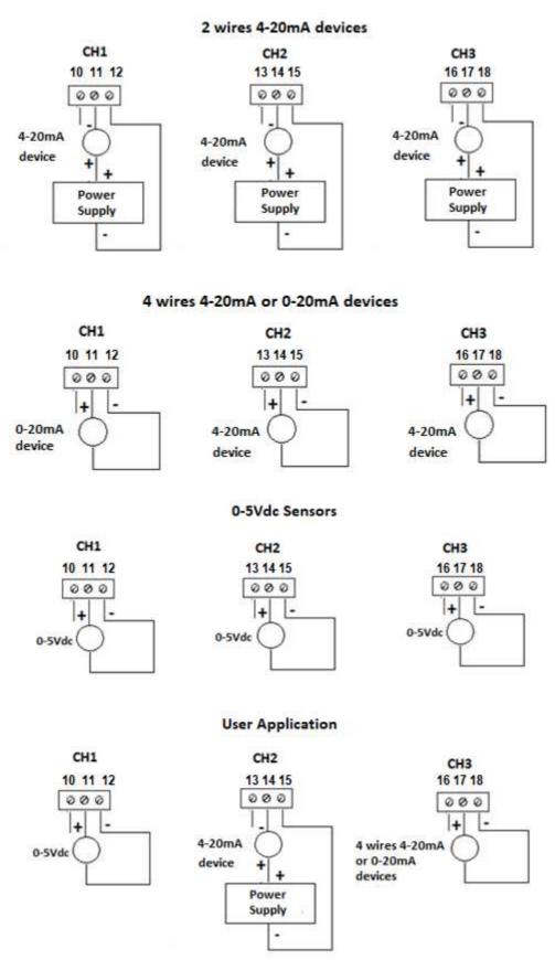
Figure 2.7 - 4-20 mA or 0-5 Vdc input connections.
