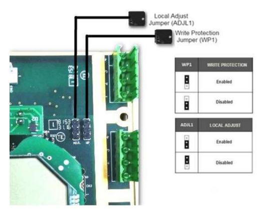
Figure 3.2 – Main board detailing jumpers.
