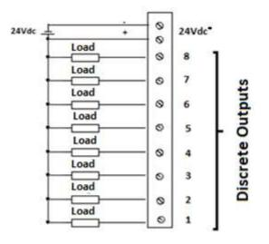
Figure 2.9 – Discrete output connections.
