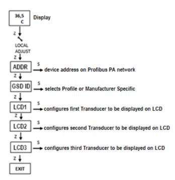
Figure 3.4 – Local adjust configuration tree.
