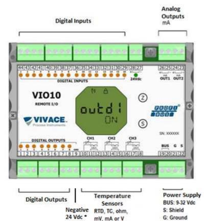
\* When using 24 Vdc external power for digital outputs (DO1 to DO8), connect the source negative to terminal 9.
